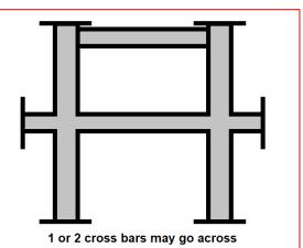
These two diagrams are a guideline to how the frame should be constructed but gusseting or triangulation is accepted.
