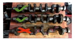
Only the crankshafts ticked green permitted twin web NO single web cranks. Internal engine parts must be as x16xe z16xe type engine and to the sizes given
