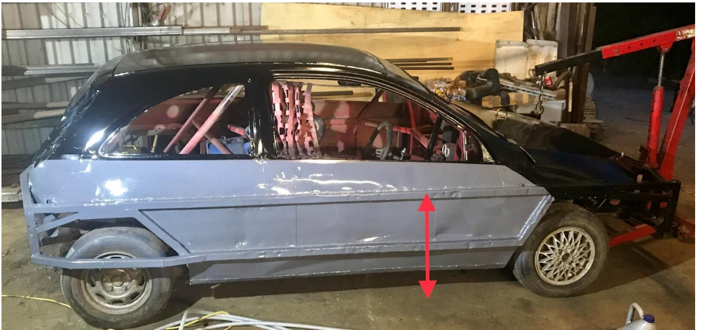
5. The bottom edge of the lower side rail must be above the top of the cars door sill
