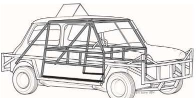
minimum size steel of 40mm x 40mm SHS or 38mm tube (minimum 3mm thick) unless stated differently.
