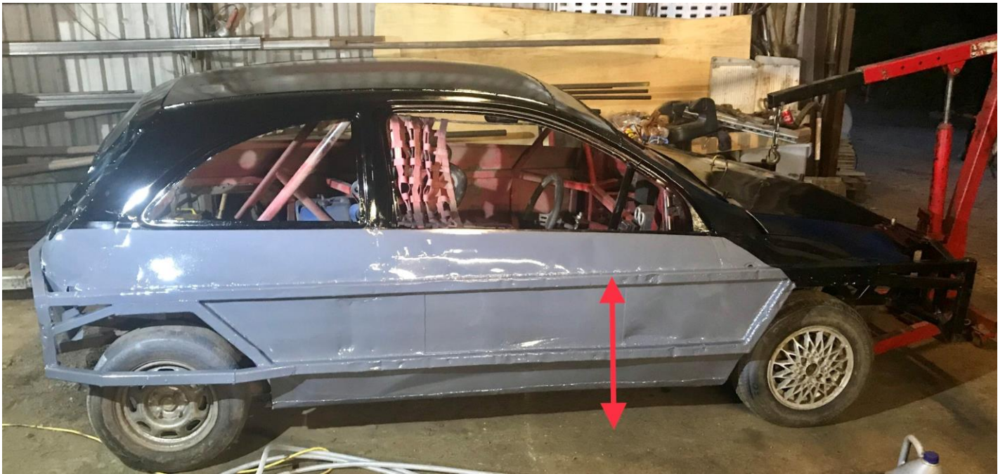
5. The bottom edge of the lower side rail must be above the top of the car door sill
